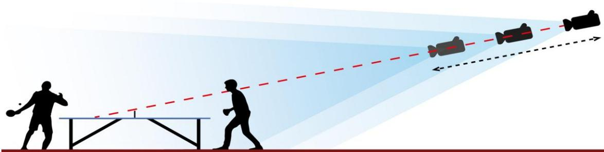
This figure acts as an example. It is mandatory that the camera is positioned in a way that the backside of the table is visible.
