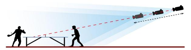
This figure acts as an example. It is mandatory that the camera is positioned in a way that the backside of the table is visible.
