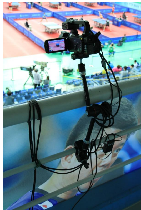
As shown in the picture below the microphones are attached to the tripod of the score cameras or the rods of the referee chair.
